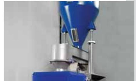
The material is fed into the Pulverizer by a vibrating dosing channel, the feeding rate is automatically adjusted based on the motors amperage and material temperature.
